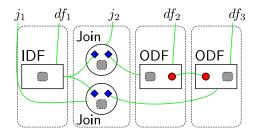
Fig. 9: Potential forbidden configuration predicate: two independent (link between the red circles) devices, regardless of location, share an input device feature. Hyper-links on IDF/ODF output/input are open but omitted for clarity.
