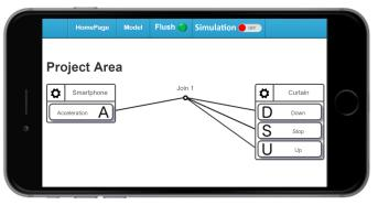
(a) IoTtalk application with two devices, *Smartphone* and *Curtain*, and four device features, *Acceleration*, *Down*, *Up*, and *Stop*. Data flows left-to-right through *Join 1* and each device feature receives the same value.
