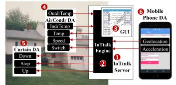
Fig. 2: The IoTtalk architecture for a smart home application.
