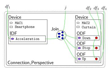
(b) Equivalent bigraph. The link connecting the three red circles represents a forbidden configuration involving the corresponding device features. Open links at the top of the diagram are used to type check the join. Details will be elaborated in Section IV.
