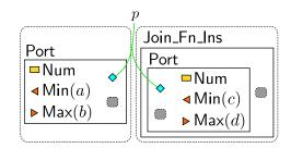
Fig. 11: Range check predicate: invalid range mapping where  $[a, b] \nsubseteq [c, d]$ .
